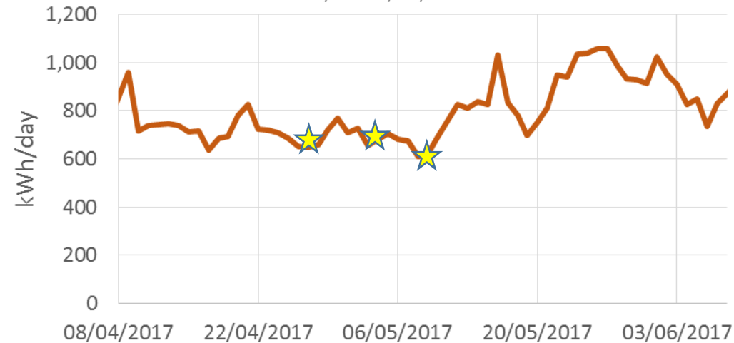
Daily PGF Process Chillers Electricity Consumption 08/04-08/06/2017
